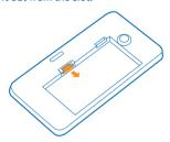
5. To remove the memory card, pull it out from the slot.
