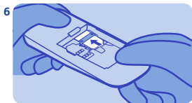
Make sure the plastic tab holds the SIM card in place.
