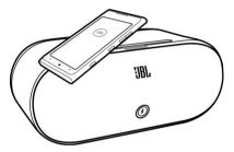
If your device supports NFC, switch NFC on, and touch the NFC area of the speaker with the NFC area of your device. The speaker connects to your device automatically. Some devices may ask for confirmation on connection. For details on NFC, see your device user guide.
