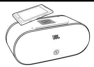
Place your phone or other compatible device on the wireless charging area on top of the speaker. The charging indicator lights turn white and flash on and off while charging. Adjust the position of your phone if the charging indicator lights blink quickly. When your phone is fully charged, the charging indicator lights go off immediately.
