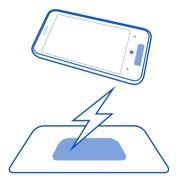
Qi works using magnetic induction, and is currently designed for devices that use 5 watts of power or less, such as mobile phones. Qi chargers and devices use the same frequency, so as long as their active areas are touching, all Qi products are compatible,
