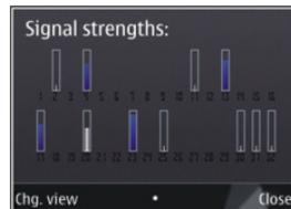
Initially, your device must receive signals from at least four satellites to be able to calculate the coordinates of your location. When the initial calculation has been made, it may be possible to continue calculating the coordinates of your location with three satellites. However, the accuracy is generally better when more satellites are found.
