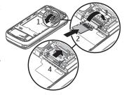
(2). Swing the card holder back in place (3), and close it at shown (4). Replace the battery cover.
