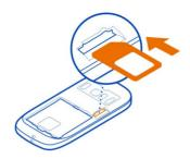
To replace the back cover, line up the locking catches and their slots, and slide 3 the cover toward the bottom of the phone.
