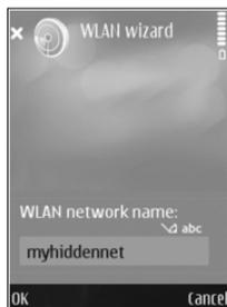
**Tip!** To make access point changes, such as changing the security key later, press
