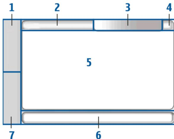
The touch screen consists of the task navigator (1), the application title area (2), the status indicator area (3), the minimise and close buttons (4), the application area (5), the toolbar (6), and the application switcher (7).
