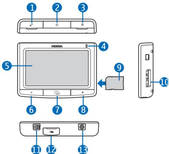
1. Cover of connector for an optional external GPS antenna
