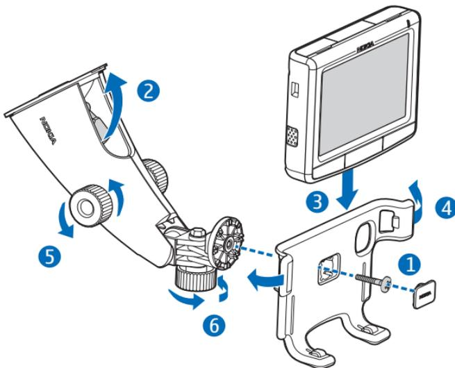
Attach the mobile holder to the mounting device using the supplied screw (1), and snap the protection plate into place. To attach the mounting device to the windscreen, carefully push the locking lever toward the cup (2). Insert the navigation device into the mobile holder (3), and press the device backwards so that the two arms of the holder lock the device in place (4). (To release the device, push the arms.) To adjust the vertical or horizontal position, use the screws (5) and (6).
