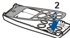
5. Place the keymat on the cut-out cover (3). Make sure that the keymat is properly in place.
