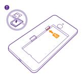
**6.** Line up the battery contacts, and put the battery in.
