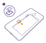
**5.** To remove the memory card, pull it out from the slot.
