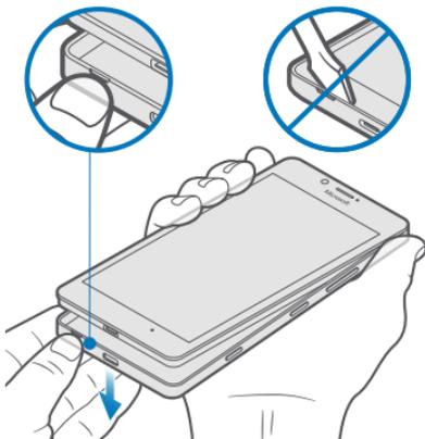
3. If the battery is in, put your fingernail in the recess on its bottom edge, and lift it out.
