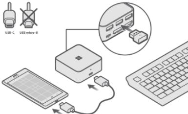
To control apps on the TV or monitor easily, connect a keyboard and a mouse to the USB connectors on the back of your accessory.
