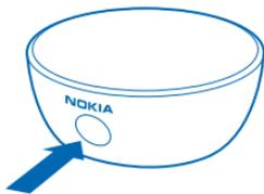
Press and hold the multifunction key for 3 seconds. If the battery is full, the battery indicator light flashes green once. If the battery indicator light is orange, you may need to charge the battery soon. If the light flashes red fast, charge the battery. When the battery is critically low, the speaker beeps repeatedly.
