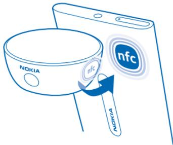
★ **Tip:** To reconnect a previously paired device, tap the NFC areas of the device and the speaker together. The speaker closes the active connection before reconnecting.
