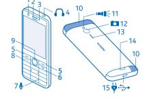
Avoid touching the antenna area while the antenna is in use. Contact with antennas affects the communication quality and may reduce battery life due to higher power level during operation.
