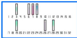
If your device has found satellites, a bar for each satellite is shown in the satellite info view. The longer the bar, the stronger the satellite signal. When your device has received enough data from the satellite signal to calculate your location, the bar color changes.
