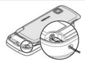
**Tip:** Attach the plectrum stylus to the device like a wrist strap.
