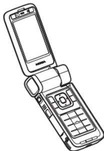
opened. The fold opens about 160 degrees, as shown in the picture. Do not force the fold to open more.
