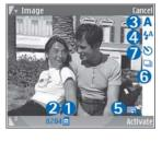
The sequence mode indicator (6) shows that the sequence mode is active. See "Take pictures in a sequence", p. 15.  The self-timer indicator (7) shows that the self-timer is activated. See "You in the picture—self-timer", p. 15.
