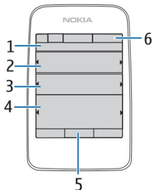
The active standby is in passive mode when the middle selection key (5) is **Menu**; you can only view content. To activate the navigation mode and scroll through the content, use the navigation key. To change the key for accessing the navigation mode, see *Enabling standby* in “*Standby mode settings*”, p. 40. When the arrow indicators are shown, you can scroll the item left and right.
