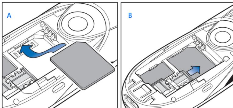
Fig. 1 Positioning and securing the memory card.
