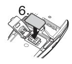
that the golden connectors on the card face the connectors on the phone.
