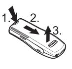
Release the cover of the SIM card holder: Press the grooved end of the cover (4). slide the cover in the OPFN direction (5)
