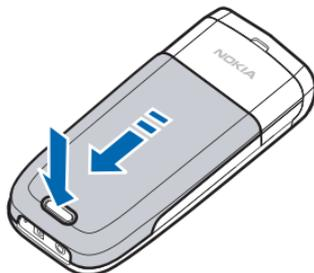
2. Slide the back cover toward the bottom of the phone and remove.
