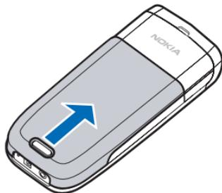
Slide the back cover toward the top of the phone until you hear a click and see the back cover release button lock into place.
