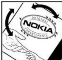
3. Scratch the side of the label to reveal a 20-digit code, for example, 12345678919876543210. Turn the battery so that the numbers are facing upwards. The 20-digit code reads starting from the number at the top row followed by the bottom row.
