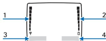
Signal strength (1)—A higher bar indicates stronger signal.
